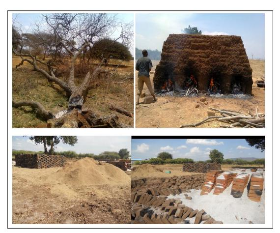
Figure 3: Fuel wood and wheat residues used for burning bricks
